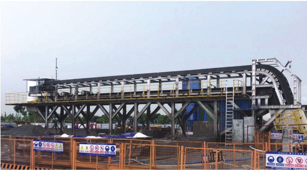
The first vertical lifting belt conveyor with a belt width of B1800 in China.
